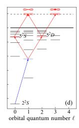
FIG. 1. Possible ionization paths. Panel (a) shows that the ejected-electron wavefunction has s-, d-, or g-symmetry (even parity) if either four red (780 nm) or two blue (390 nm) photons are absorbed. The remaining panels are cases where two red and one blue photon are absorbed, thereby leading to continuum states of p- or f-symmetry (odd parity).
