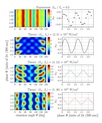
FIG. 4. Left column: raw measured (top) and calculated relative phase  $\Phi$  traces of the PADs for selected peak intensities and intensity ratios. Right column: Corresponding angle-integrated asymmetry parameter  $A_{LR}$  for each trace.
